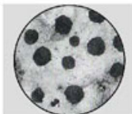
● Material: ductile iron FCD-60.
