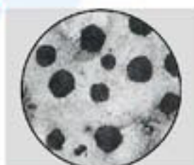
Microphotograph for ductile cast iron
