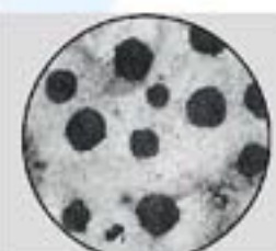
Microphotograph for ductile cast iron
