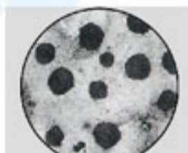
Microphotograph for ductile cast iron
